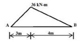
The magnitude of the concentrated load in kN is \_\_\_\_\_
