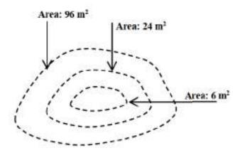
The contour interval is 1 m. Using prismoidal method, the volume of the earth needed to fill the land depression is m<sup>3</sup>.
